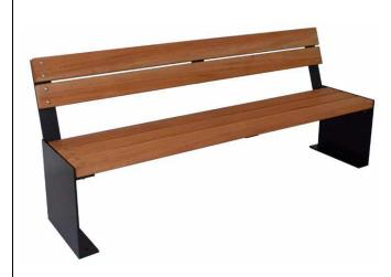
Bench Amburgo with backrest has a structure in galvanized and powder coated steel, composed by two supports in laser-cut steel sheet 8 mm thick, on which are welded drilled base plates for the fixing at the ground with bolts.
